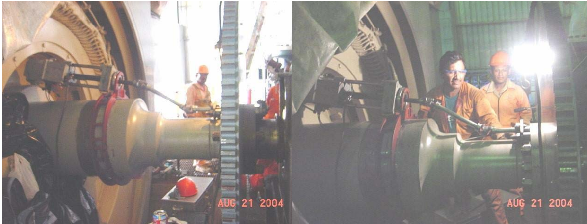
York End Mount and offset bar drive with custom mounting fixture
